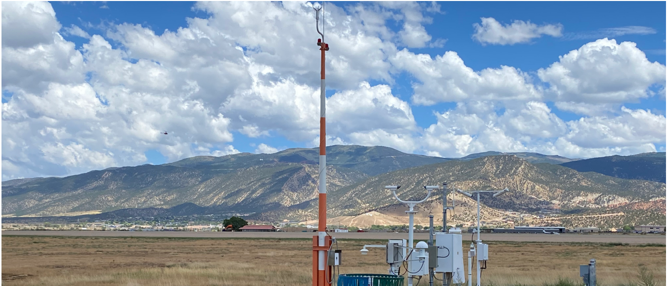
Figure 4.19: Automated Surface Observing System
